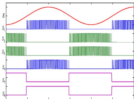
Fig.5. Modulation Scheme for gate drive signals with unity power factor.
