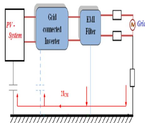
Fig.1. Transformerless PV system
