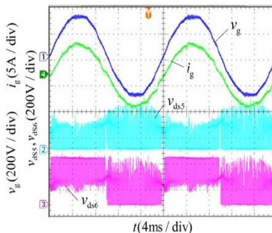
Fig.12. Voltage stress on S5 and S6 of Drain–source voltages
