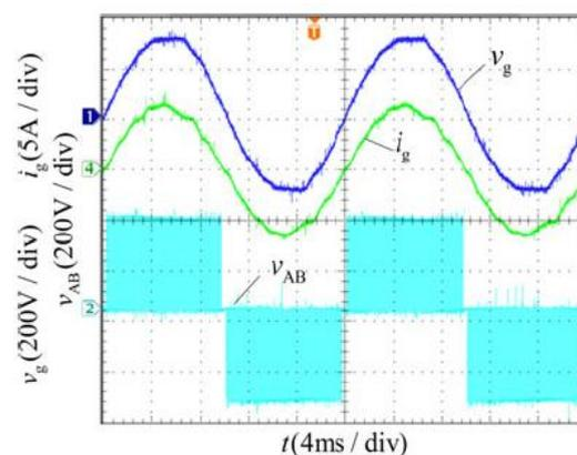
Fig.13. DM characteristic of H6 topology.
